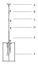
2) Secure assembled fixture body and stem to canopy
