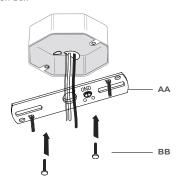
5) Connect the copper wire from canopy (A) to the mounting bracket (AA), securing with pre-installed ground screw.
