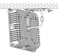
**E)** Secure the fixture to the mounting plate by fastening the screws on both sides of the luminaire.
