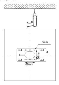
**C)** Install the anchors and secure mounting plate to the ceiling.
