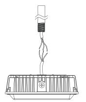
B) Fasten the luminaire to the 3/4" NPT stem.
