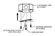
B) Feed power cord through cord grip cap, the canopy, then through cord grip base, and make adjustments to overall suspension length.
