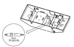
**D)** Align clips and push housing directly onto the backplate. Apply continuous AC power and press "TEST" button to check the light.
