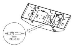
C) Align clips and push housing directly onto the backplate. Apply continuous AC power and press "TEST" button to check the light.
