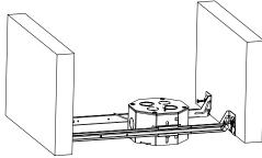
B) Secure hanger bar to wood joist with rivet.
