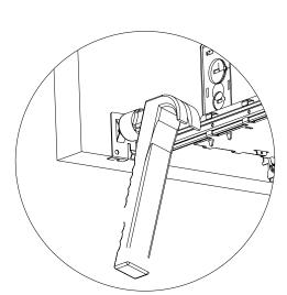
C) Adjust the channels as desired, and secure to joists using screws.
