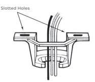
NO MOVEMENT SHOULD OCCUR BETWEEN THE MOUNTING BRACKET AND THE ELECTRICAL JUNCTION BOX.
