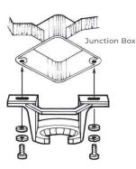
B) The mounting bracket has slotted holes to enable it to move sideways for proper alignment. Make sure the mounting bracket is centered over the electrical junction box and that it is securely attached. **C)** Loosen the two canopy mounting screws on the underside of the mounting bracket halfway. This will allow for easier installation of the ceiling canopy.
