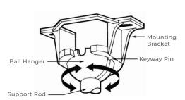
**C)** Trim the lead wires, leaving about six inches of each wire extending from the support rod.
