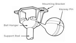
B) Lift the fan and place the ball hanger in the center of the mounting bracket with the keyway pin inserted into the keyway on the ball hanger. Turn the fan left and right slightly to make sure it is securely aligned on the bracket with the keyway pin in the keyway.
