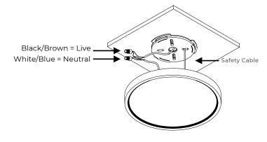
E) Match the alignment arrows as indicated on the mounting plate and the luminaire body. Install the luminaire body to the mounting plate by rotating clockwise.
