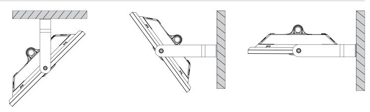
For the above installation options, secure the fixture with safety ropes.
