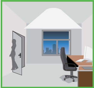
The light will dim to a stand-by after hold-time and stays on selected minimum dimming levels.
