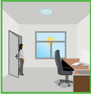
The light will not switch on when natural light is present, even if there is motion detected.
