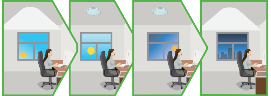
The light output will regulate according to the level of natural light present.
