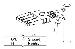
C) Install the bracket cover and tighten the screws. The luminaire aiming angle is adjustable.
