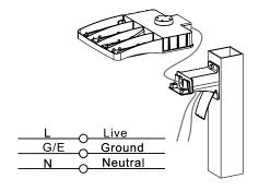
C) Install the bracket cover and fasten the screws. Installation complete.
