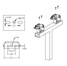
B) Install the luminaire onto the bracket and fasten with provided screws.
