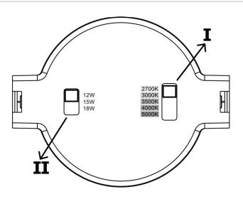
**SWITCH I** Selectable CCT 2700K / 3000K / 3500K / 4000K / 5000K SWITCH II Selectable Power •4-inch Selectable: 8W / 10W / 12W •6-inch Selectable: 12W / 15W / 18W
