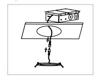
**D)** Install the fixture to ceiling surface, as shown below.
