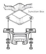
B) The mounting bracket has slotted holes to enable it to move sideways for proper alignment. Make sure the mounting bracket is centered over the electrical junction box and that it is securely attached.
