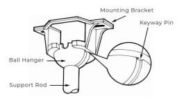
B) Lift the fan and place the half ball in the center of the mounting bracket with the keyway pin inserted into the keyway on the ball. Turn the fan left and right slightly to make sure it is seated on the bracket with the keyway pin in the key way.
