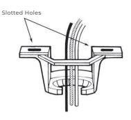
NO MOVEMENT SHOULD OCCUR BETWEEN THE MOUNTING BRACKET AND THE ELECTRICAL JUNCTION BOX.
