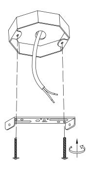
**C)** Make wiring connections. Secure canopy to mounting bracket using provided screws. Installation is complete.
