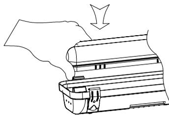
C) Attach V-Hook to the suspension chains.
