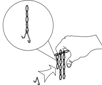
D) Attach bracket to the back of the fixture.
