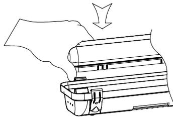
C) Screw the mounting bracket into the ceiling with provided screws. Applying minimal pressure, snap fixture into secure mounting brackets.
