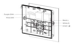
7) Connect the two low voltage wires from driver to LED PCB.
