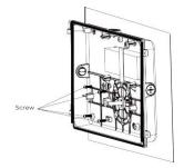
6) Make wiring connections and place in back box.
