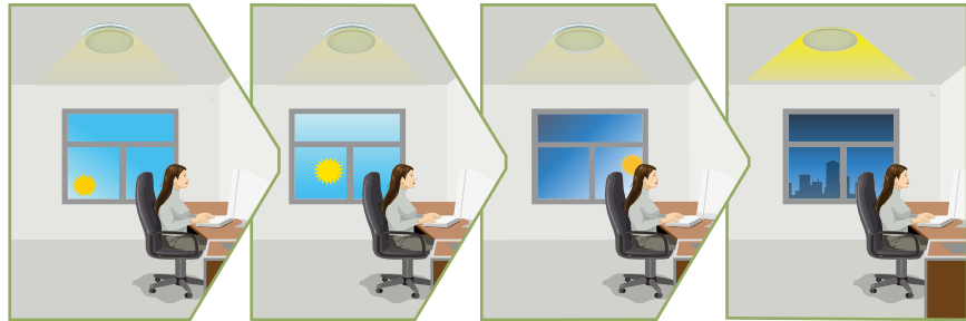
The light turns on at full or dims to maintain lux level. The light output regulates according to the level of natural light available.
