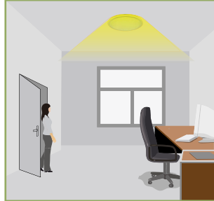
With insufficient natural light, the sensor switched on the light automatically when presence is detected.
