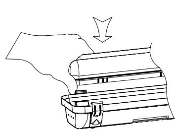
**C) Screw the mounting bracket into the ceiling with provided screws. Applying minimal pressure, snap fixture into secure mounting brackets.**
