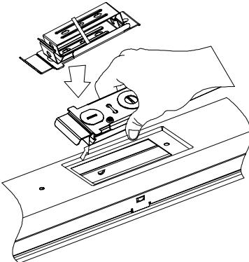
**C)** Screw the mounting bracket into the ceiling with provided screws. Applying minimal pressure, snap fixture into secure mounting brackets.
