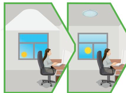
The light output will regulate according to the level of natural light present.
