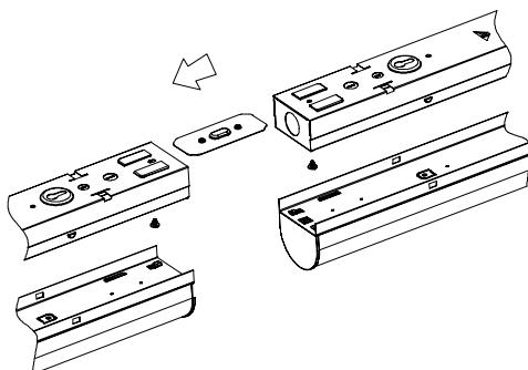
**C**) Reattach wireway cover assembly to the housing assembly.
