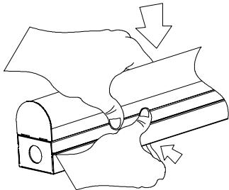
**B**) Use the hard to adjust CCT in Dip Switch if needed. Standard CCT: 4000K
