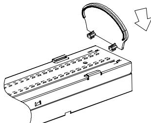
**D**) Replace the lens on the fixture.
