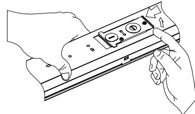
**B)** Remove the mounting brackets from underside of outlet plate.
