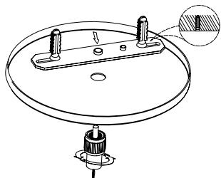
**E)** Install the aircraft cable gripper.
