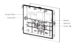
7) Connect the two low voltage wires from driver to LED  $\hspace{-0.1cm}$  PCB.
