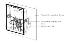
5) Use screws to secure the fixture base to the back box.
