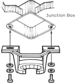
**B)** The mounting bracket has slotted holes to enable it to move sideways for proper alignment. Make sure the mounting bracket is centered over the electrical junction box and that it is securely attached.
