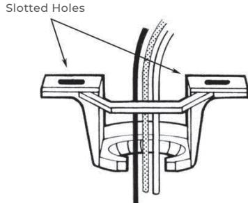
**C)** Loosen the two canopy mounting screws on the downside face of the mounting bracket. Back them out about half way. This will allow for easier installation of the ceiling canopy later.
