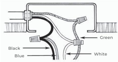
**B)** Fold the connected wires push them up inside the electrical junction box with the BLACK and BLUE wires to one side and the WHITE and GREEN to the other side. Make sure the wire nuts do not come loose during operation.
