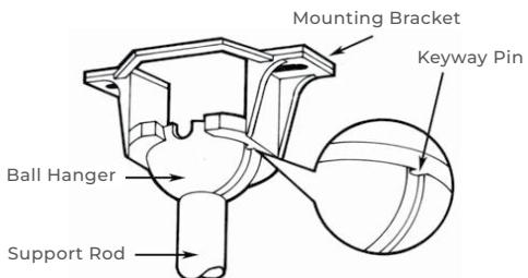
**B)** Lift the fan and place the half ball in the center of the mounting bracket with the keyway pin inserted into the keyway on the ball. Turn the fan left and right slightly to make sure it is seated on the bracket with the keyway pin in the key way.
