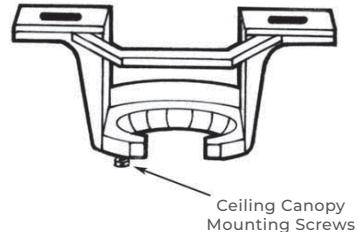
**NO MOVEMENT SHOULD OCCUR BETWEEN THE MOUNTING BRACKET AND THE ELECTRICAL JUNCTION BOX.**
